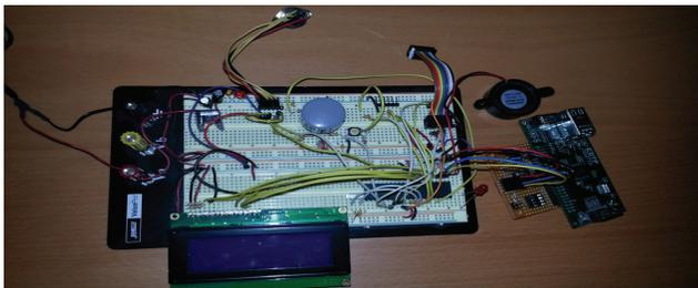
*Prototype with 4x20 LCD display and Ethernet adapter.
