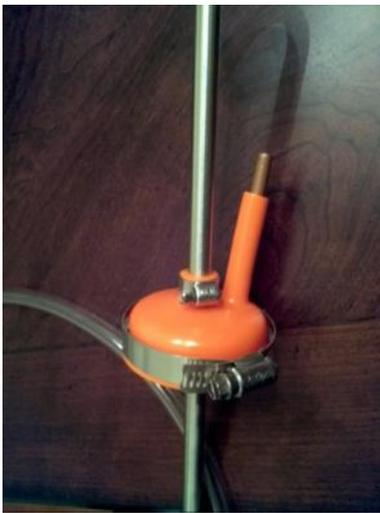
**Tip:** I have found that the orange carboy caps do not always form an air-tight fit without a little help. I just use a hose clamp as a collar to lock it down on the mouth of the carboy. As you may notice in the photo, I have to do the same thing with the port for the racking cane but that has more to do with where I cut the port.
